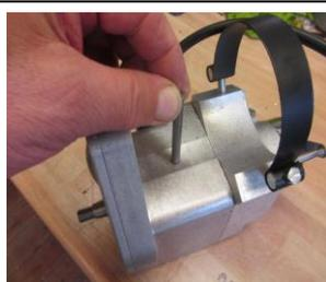
1. Turn the magneto shaft until the engraved arrow on the end of the shaft is pointing down towards the base (figure 1.)
