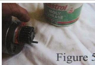
10. The black wire cuts the magneto when earthed. Connect this wire to a switch or kill button for stopping the engine.
