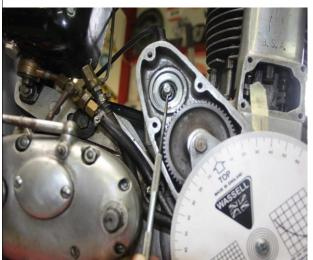
Dot on shaft at bottom. There will also be an arrow engraved on end of the shaft pointing to the dot so you can check the orientation when the gear and nut is fitted.
