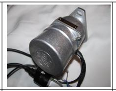
3. Remove the brass timing hole screw from the BT-H magneto
