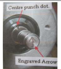
4. Turn the magneto shaft until the arrow is a at the top pointing up towards the timing hole.
