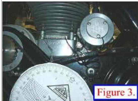
7. Fit your timing pinion and tighten the nut. We recommend 15 ft-lbs if you have a torque wrench.
