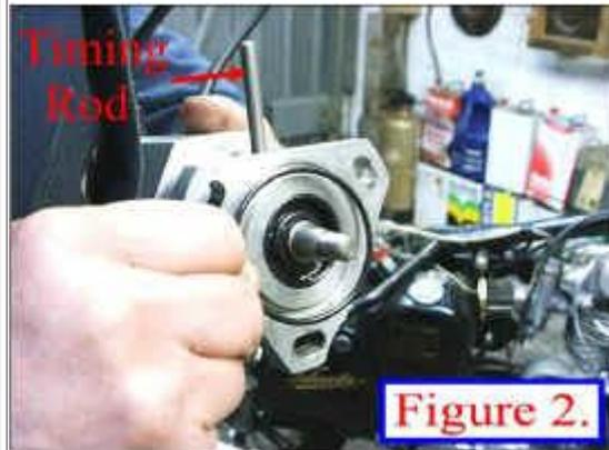
5. Fit the magneto in place on the three studs. The fixing holes are slotted to allow minor adjustments to be made to your ignition timing without any dismantling. We suggest that you set the holes to the centre of the slots before tightening.
