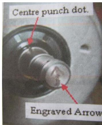
4. Turn the magneto shaft until the arrow is at the top pointing up towards the timing hole.
