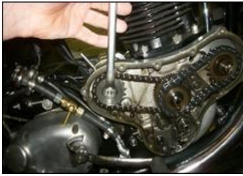
8. Replace the timing pinion and torque the nut to 12/15 ft/lbs maximum.
