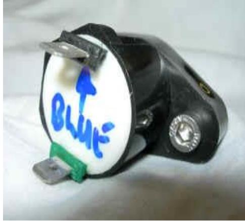
11. Connect the wiring referring to the picture of the HT coil. The blue wire goes to the black spade on the H.T. coil. The wire with the yellow tag goes to HT coil of the cylinder that you timed the ignition on. The brown wire goes to the green spade. The coil does not need to be earthed to the frame. The black wire is for the cut out. It cuts the ignition when earthed. If you do not use this cut out wire make sure that the end is well insulated so that it can not inadvertently stop the engine.
