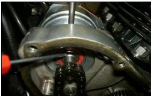
4. Fit the "O" ring into the groove on the flange of your new magneto using a little grease to retain it.
