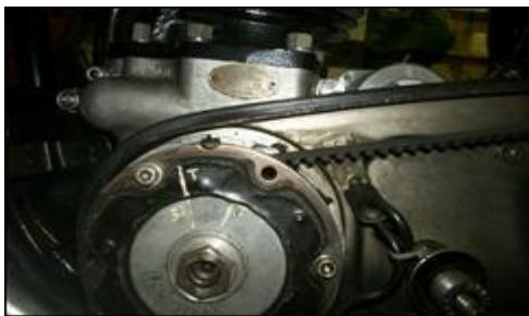
7. Set the crankshaft to the **FULL ADVANCE\*** position (inches, mm or degrees) BTDC on the left hand cylinder on the compression stroke. We have found that 2 or 4 degrees less advance may work better with modern fuels.
